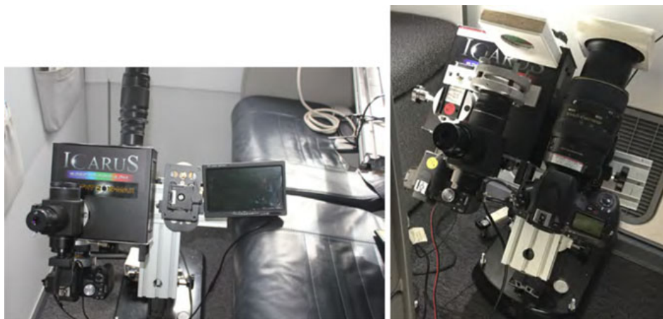
Figure 19. Collaborative equipment sent aloft on the chartered 787-9 airplane. The NIR spectrograph and the telephoto lens are on a motorized azimuth mount. The image to the left was taken during a pre-eclipse test flight.
